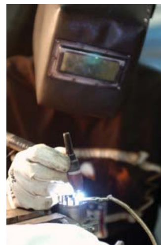
Tungsten inert Gas Welding of Stainless and Aluminum
